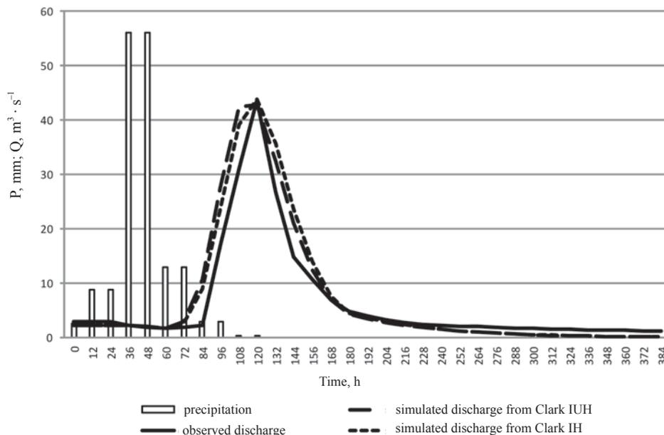
Fig. 2. Comparison of observed and SUH hydrographs for case study (P – precipitation, Q – discharge)
