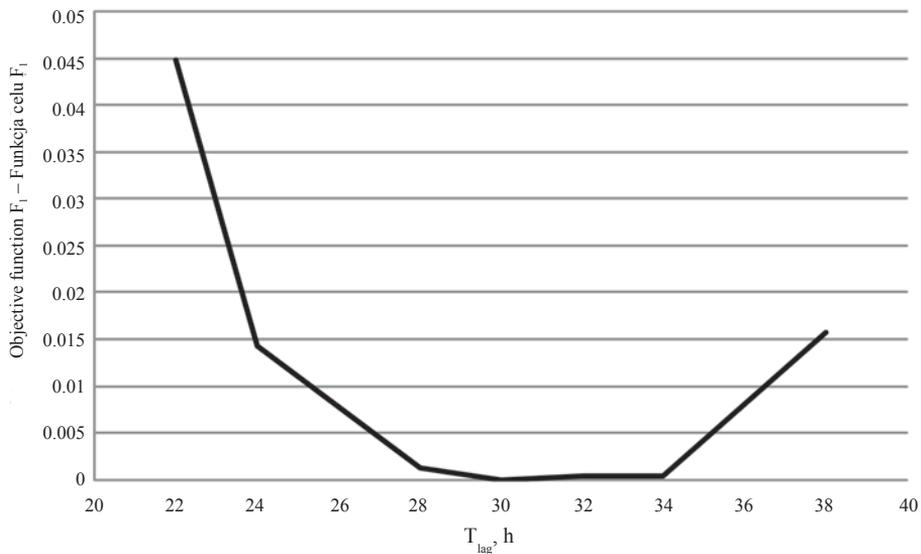
Fig. 3. Optimum  $T_{lag}$  yielded by different values of objective function  $F_1$
