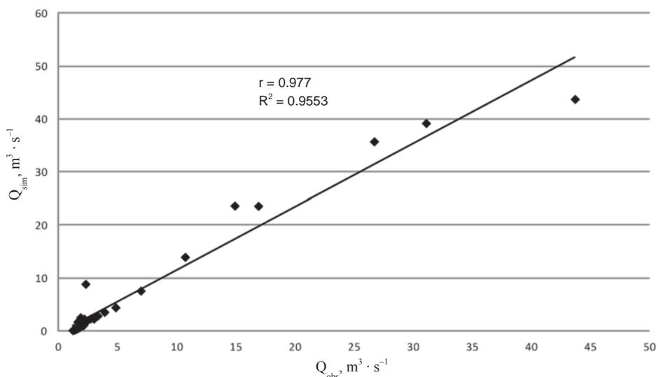
Fig. 4. Observed versus Snyder UH-simulated flows
