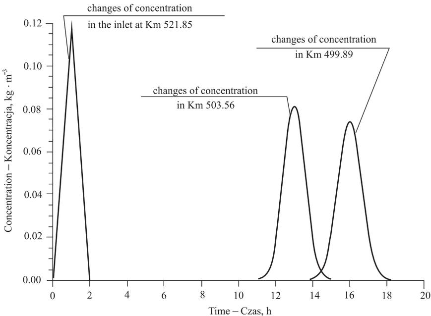
Fig. 2. Typical results of admixture transport simulation; parameters: bottom state (1), discharge  $20 \text{ m}^3 \cdot \text{s}^{-1}$ , water level 117.0 m a.s.l., maximum concentration  $0.12 \text{ kg} \cdot \text{m}^{-3}$ , penetration time 65 s, dispersion estimated from Elder formulae
