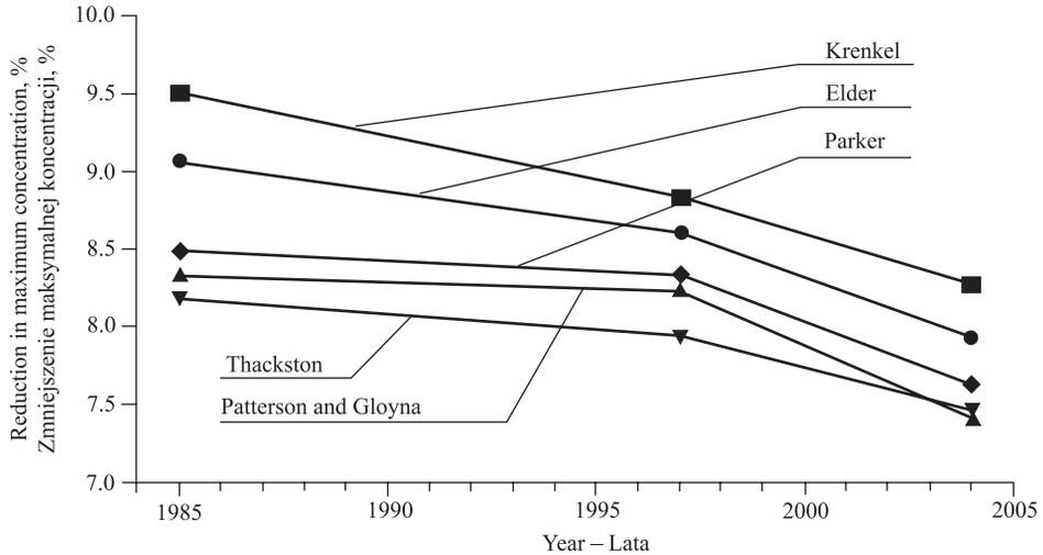
Fig. 3. Changes in the maximum concentration of potential dissolved substance in the reach under investigation in percentages for the discharge  $20 \text{ m}^3 \cdot \text{s}^{-1}$ , water level 117.0 m a.s.l., penetration time 65 s and maximum concentration in the inlet  $0.12 \text{ kg} \cdot \text{m}^{-3}$
