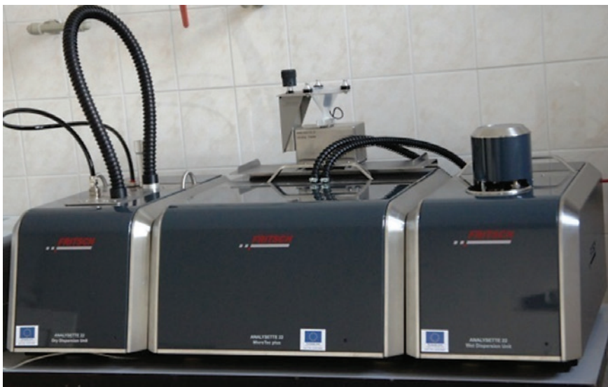
Fig. 1. ANALYSETTE 22 MicroTec plus (left to right): dry dispersion unit, measuring unit, wet dispersion unit (Photo E. Kondrlová)
