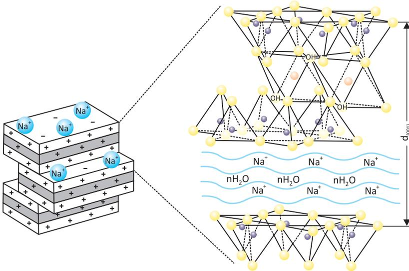
Fig. 1. Sodium bentonite structure [www.technologie-budowlane.com]
