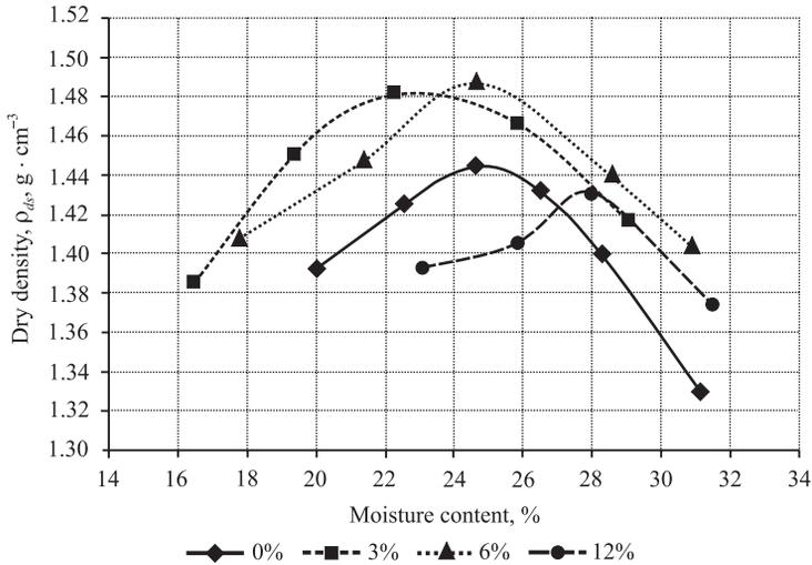
Fig. 3. Proctor curves for bottom sediments and their mixtures with bentonite
