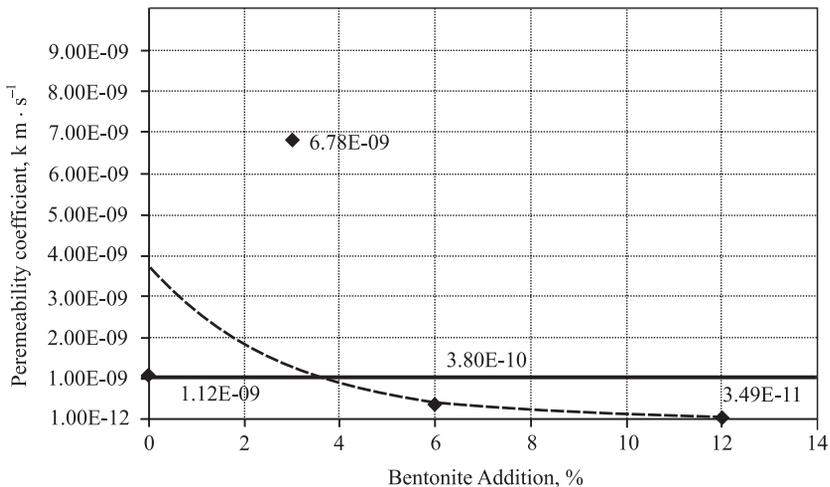
Fig. 4. The influence of bentonite addition on the permeability of sediments in relation to Polish Regulation requirements [Rozporządzenie... 2003]
