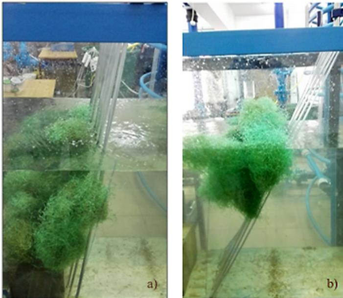
Fig. 4 a) Flat rectangular bars inclined to the channel bottom at an angle of 80° for 0.5 kg debris weight, b) Cylindrical bars inclined to the channel bottom at an angle of 80° for 0.5 kg debris weight
