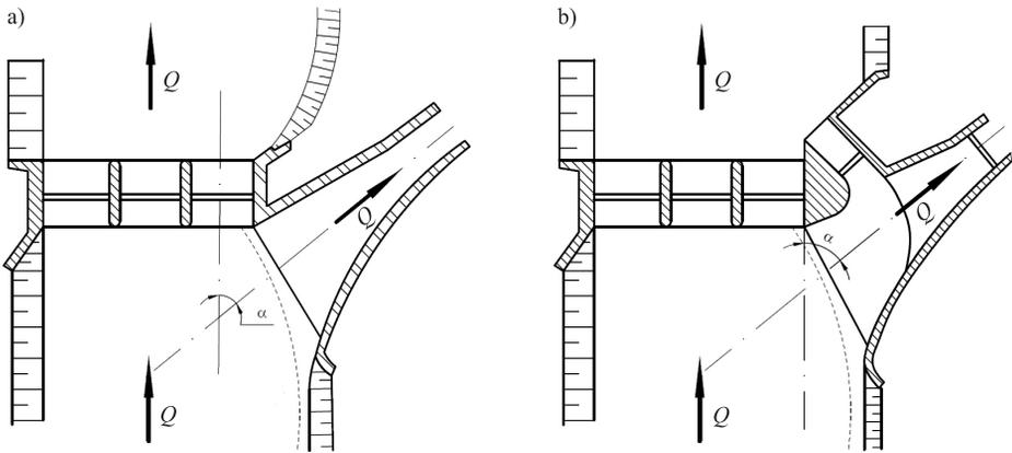
Fig. 2. The location of intakes (inlets) to the energy channel on a straight stretch of river a) with flushing through a weir, b) with a separate flushing duct [Balcerski 1969].
