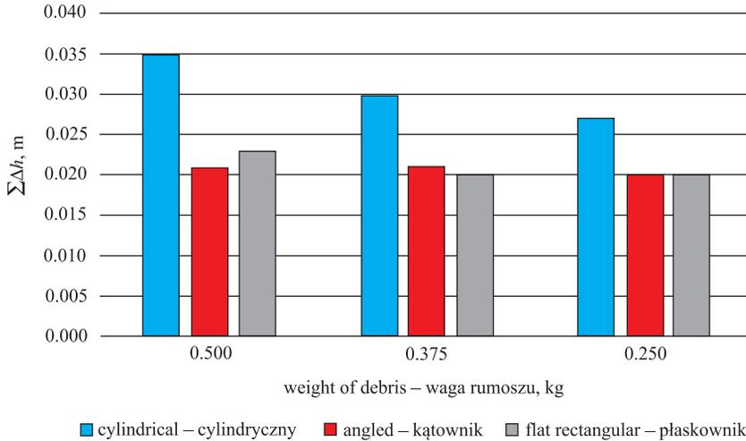
Fig. 7. Losses due to clogging trash racks with plant debris for variously shaped bars inclined at an angle of 80° with different plant debris weights
