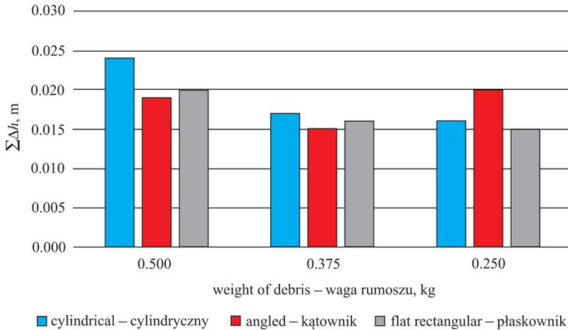
Fig. 5. Losses due to clogging trash racks with plant debris for variously shaped bars inclined at an angle of  $30^\circ$  with different plant debris weights
