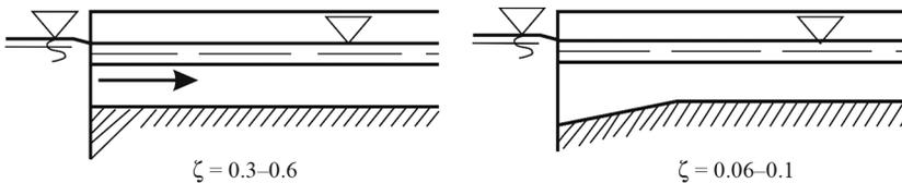
Fig. 3. Typical inlet shapes to intakes and corresponding loss coefficients – open channels [Balcerski 1969].
