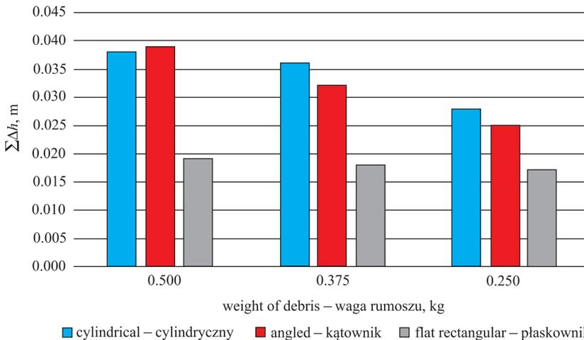
Fig. 6. Losses due to clogging trash racks with plant debris for variously shaped bars inclined at an angle of  $60^\circ$  with different plant debris weights
