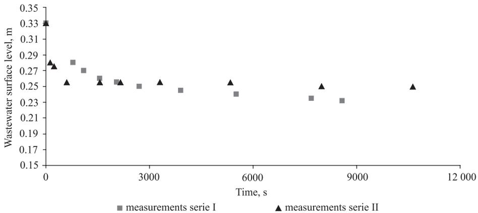
Fig. 2. Wastewater level surface – highly changeable flow-conditions experiment
