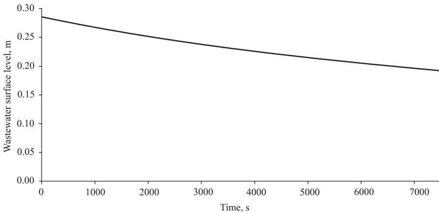
Fig. 6. Verification of slightly changeable flow-conditions mathematical model by the experiment data set (porosity: 0.53 and bio-grains diameter:  $1.66 \pm 0.01 \mu\text{m}$ ).
