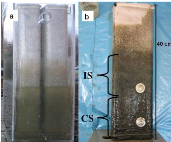
Fig. 1. Research reactor – front view (a), continuously (CS) and intermittently (IS) saturated regions of filter (b)
