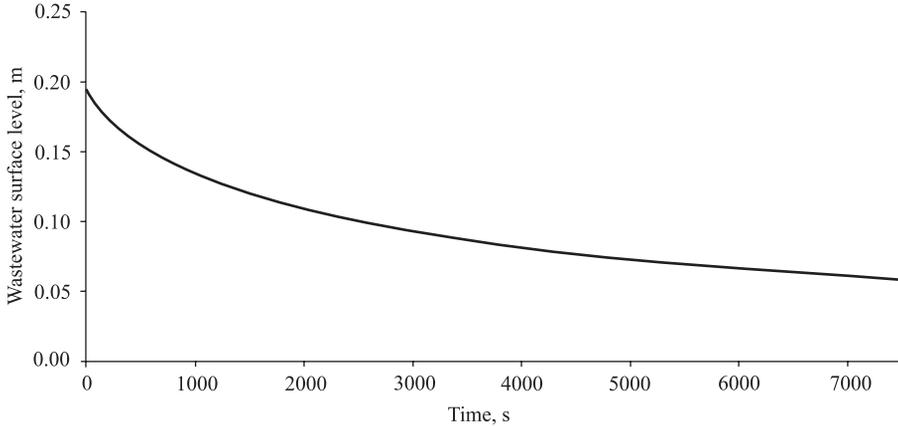
Fig. 5. Verification of highly changeable flow-conditions mathematical model by the experiment data set (porosity: 0.53, 0.57, 0.74 for zones 1–4, 5–7 and 8–10, respectively and bio-grains diameter:  $1.66 \pm 0.01 \mu\text{m}$ ).
