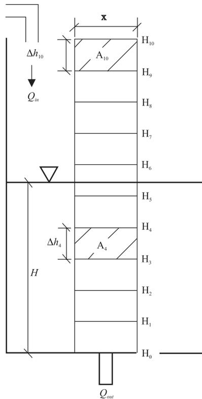
Fig. 4. Hydraulic model assumptions and the basic model parameters
