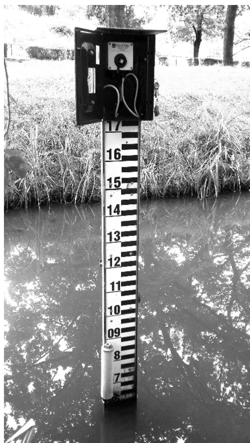
Fig. 2. Gauge Station upstream of the Staw Wyścigi (Pond), optical turbidity sensor with data recorder and gauge staff
