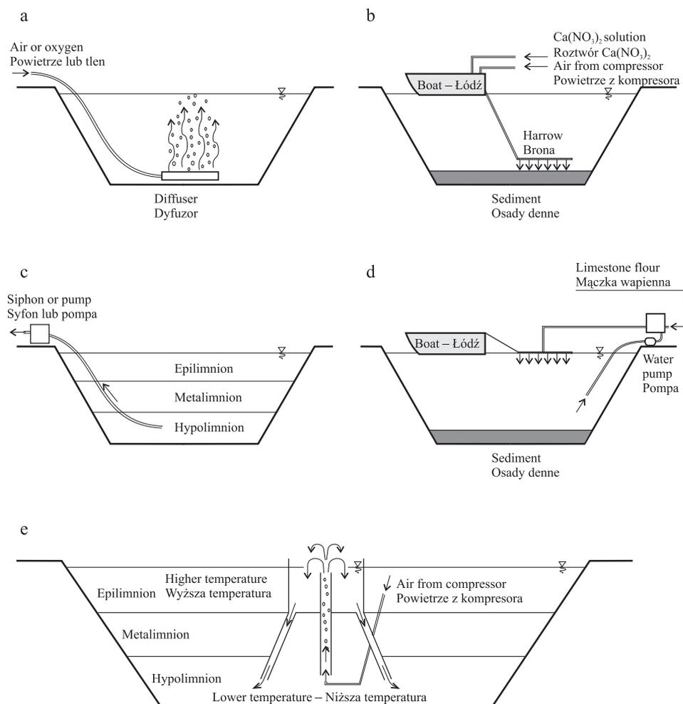
Fig. Schemes of some reclamation methods: a – hypolimnetic aeration with artificial destratification, b – sediment oxidation (nitrate treatment), c – removal of water from hypolimnion, d – lime treatment, e – hypolimnetic aeration without disturbing the temperature (based on: Kajak [1998], Perrow and Davy [2002])
